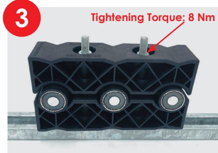
Alternating, tighten nuts with an appropriate torque wrench. Do not use self-securing/self-locking nuts, this prohibits a defined tightening torque. Tightening Torque for more rows: 8 Nm
