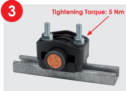
Alternating, tighten nuts with an appropriate torque wrench. Do not use self-securing/self-locking nuts, this prohibits a defined tightening torque.
